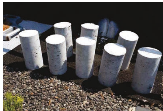
Concrete test cylinders on the green roof of Colburn Laboratory, where they are exposed to normal weather conditions.
