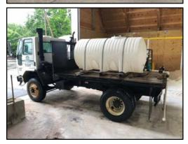
also added to the truck. The truck performed exceptionally well when running the brine application rate testing (50 gallons per lane mile at 20 MPH).
