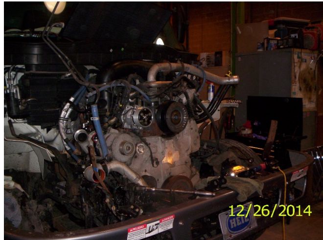
Cooling fan bearing repair on rear loader
