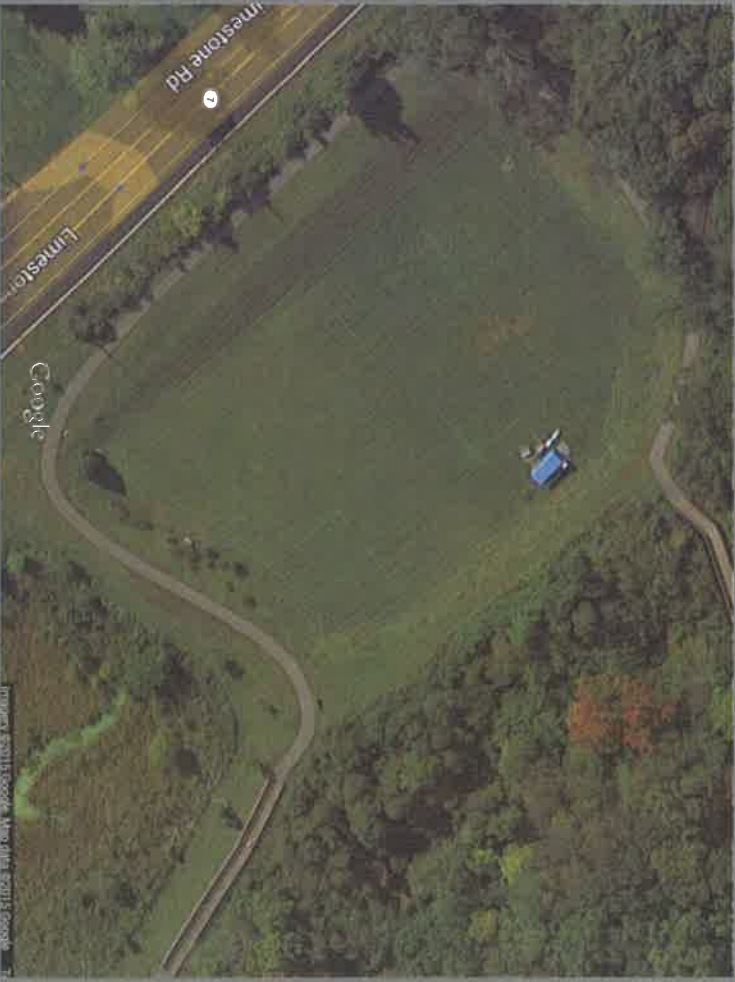
Hockessin Athletic Club – Soccer Fields Within Stormwater Detention Basin
